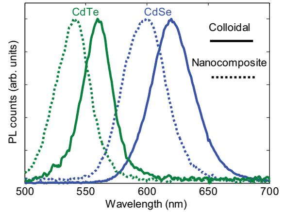
Fig. 3. Photoluminescence spectra of CdSe and CdTe QDs incorporated in the colloidal solution and in the PMMA nanocomposite.
