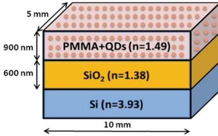
Fig. 1. Structure of the fabricated planar waveguides (not to scale).
