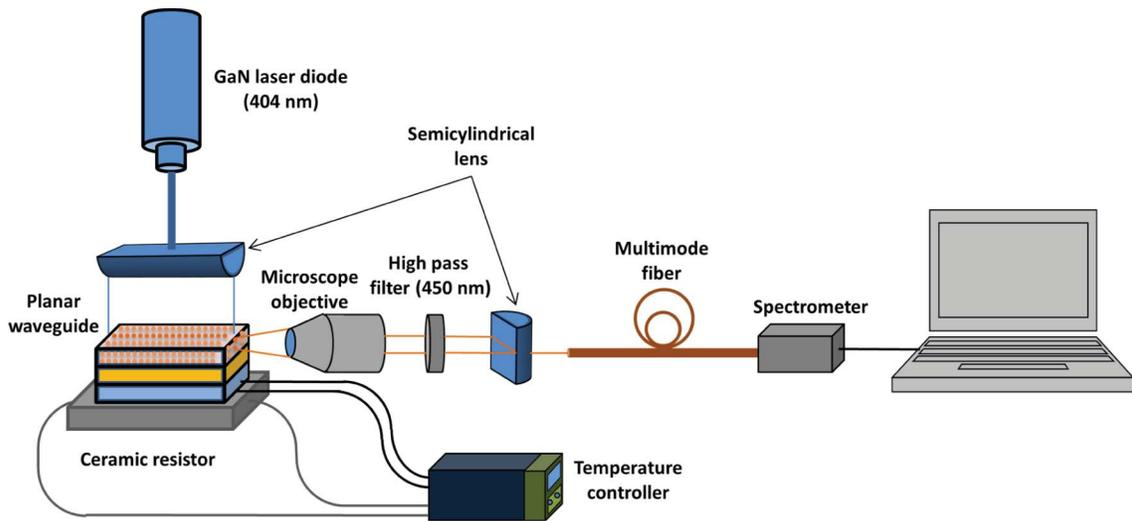
Fig. 4. Experimental setup carried out in order to perform temperature experiments with CdSe-PMMA and CdTe-PMMA waveguides.
