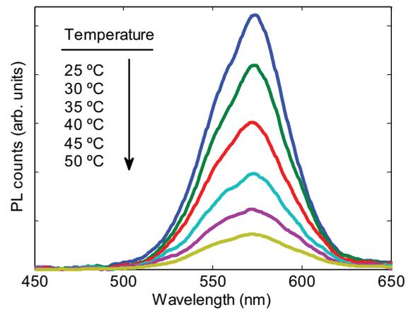
Fig. 5. Photoluminescence spectra recorded from the CdSe-PMMA waveguide at each setting temperature.
