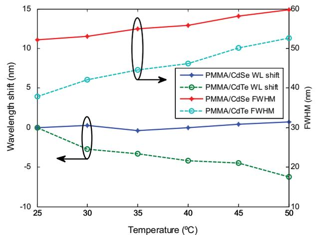
Fig. 6. Temperature dependence of wavelength shift and FWHM of PL spectrum.
