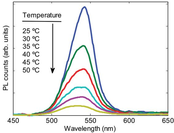
Fig. 7. Photoluminescence spectra recorded from the CdTe-PMMA waveguide at each setting temperature.
